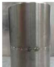
Pipe butt weld Ø 31,75 x 2 mm.
