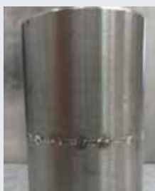
Pipe butt weld Ø 31,75 x 2 mm.
