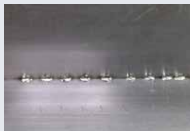
Corner spot welding thickness 0,6 mm
