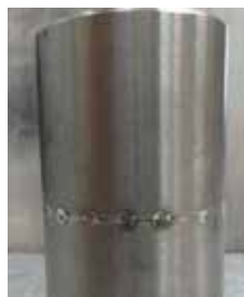
Pipe butt weld Ø 31,75 x 2 mm.
