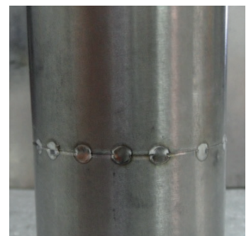
Pipe butt weld Ø 31,75 x 2 mm
