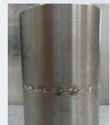
Pipe butt weld Ø 31.75 x 2 mm
