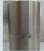
Pipe butt weld Ø 31.75 x 2 mm
