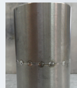
Pipe butt weld Ø 31.75 x 2 mm
