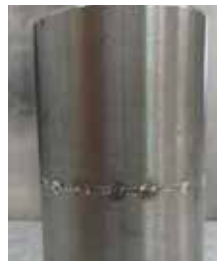
Pipe butt weld Ø 31.75 x 2 mm
