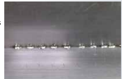
Corner spot welding thickness 0,6 mm
