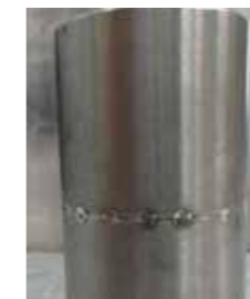
Pipe butt weld Ø 31.75 x 2 mm
