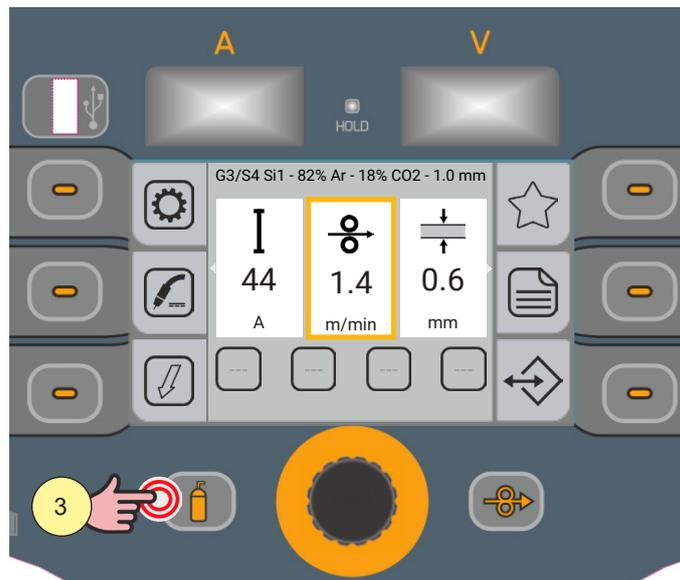
3. Close the gas solenoid valve by pressing and releasing the [GAS] key. The solenoid valve closes automatically after 30 seconds.
