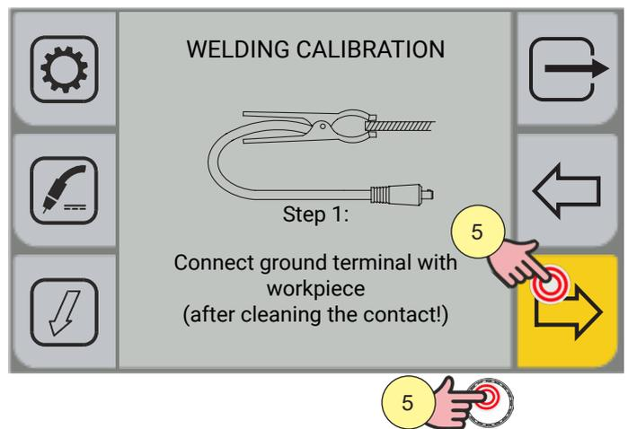
4. Press the encoder key or the [NEXT] key, or the torch trigger to confirm, or the [Wire forward] key
