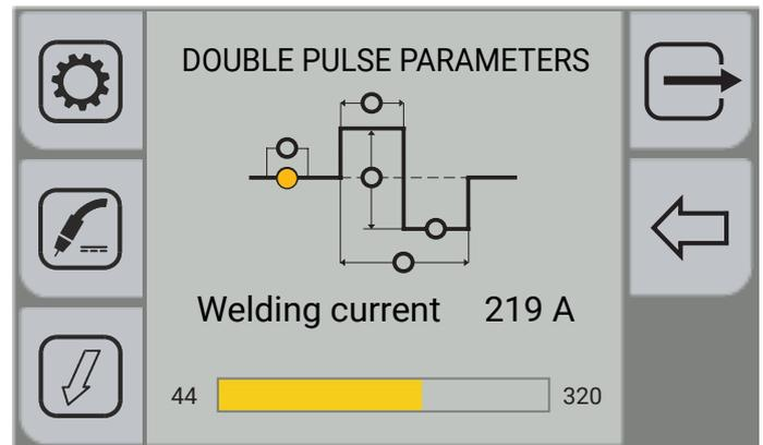
4. Turn the encoder to select the parameter to be modified.
