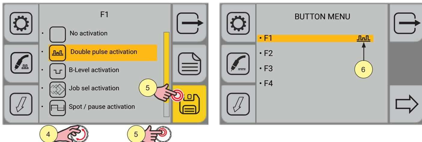
4. Turn the encoder to select the desired function.
