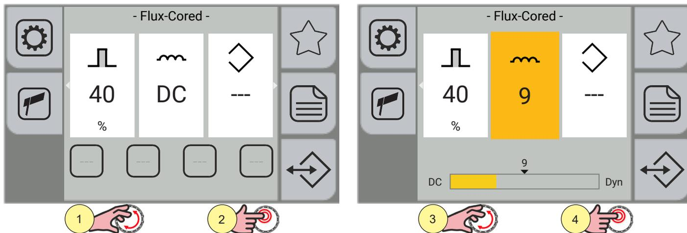
1. Turn the encoder to select the parameter to be modified.
