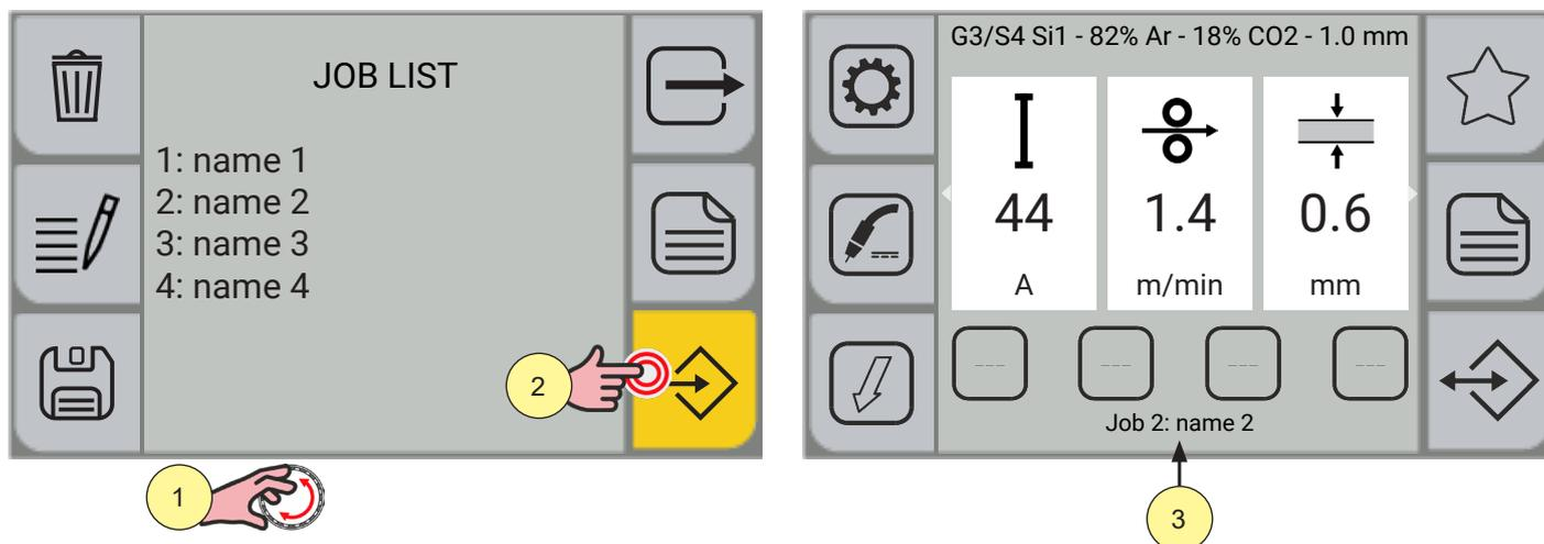
1. Select the JOB to be loaded using the encoder.
