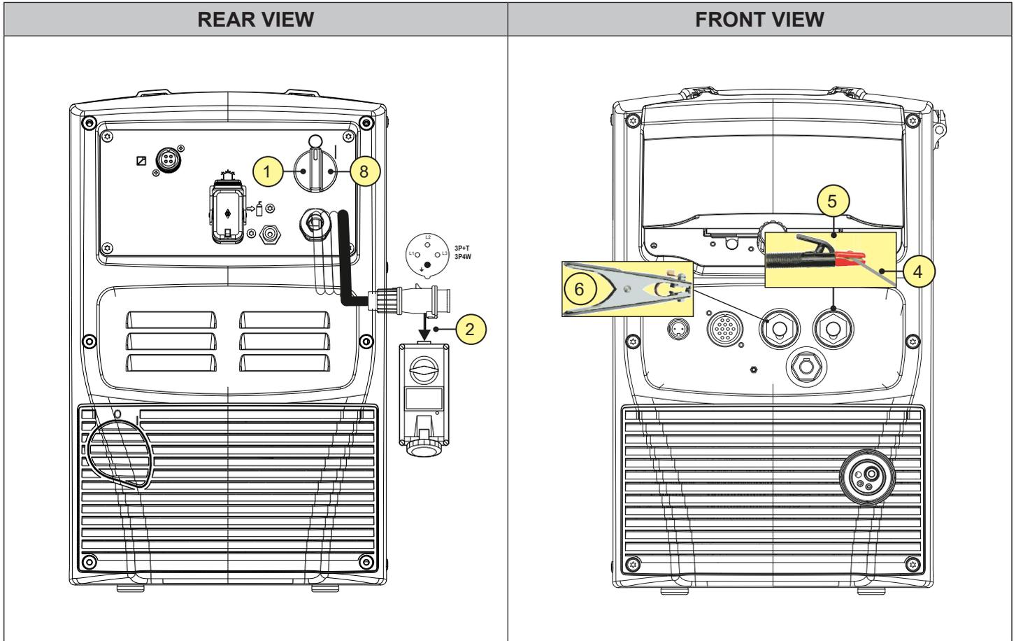
1. Place the current generator switch in position “O” (equipment off).
