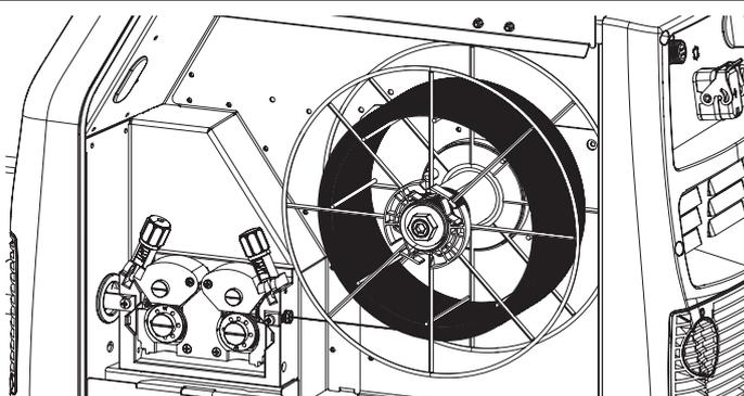
4. Check that the feed rolls are suitable for the wire gauge.
