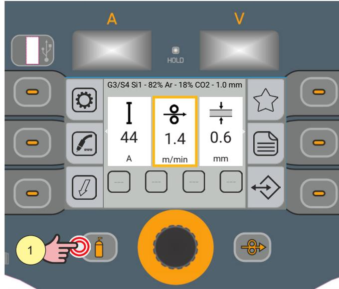
1. Open the gas solenoid valve by pressing and releasing the [GAS] key.
