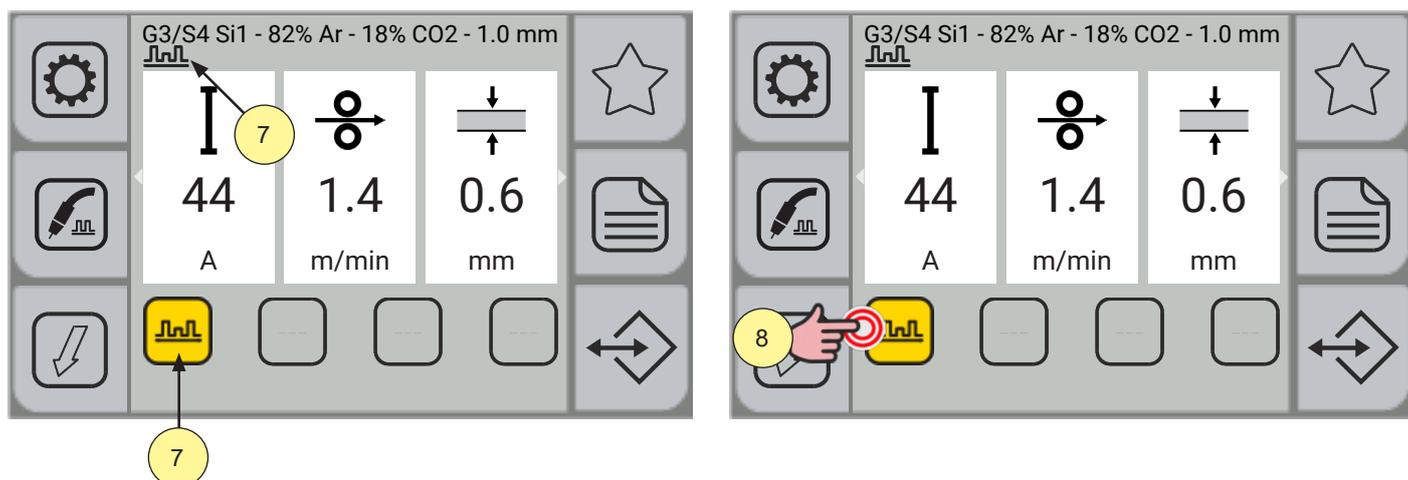
7. Once the desired function is associated with the [SHORTCUT] key, the function icon is displayed both in the [BUTTON] menu and on the key in the main screen.
