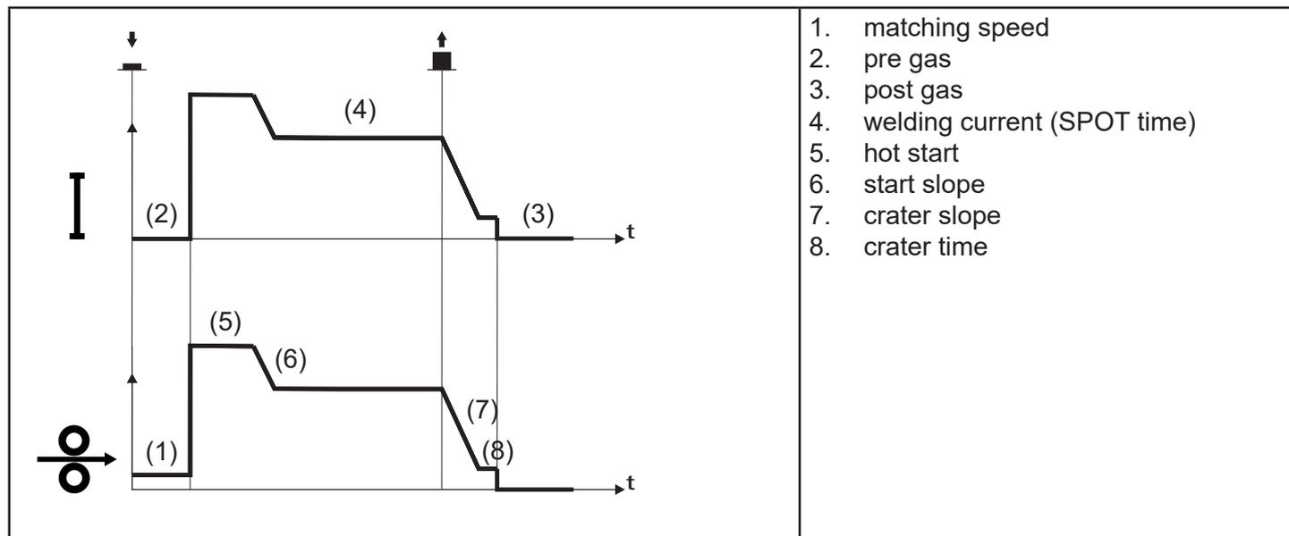
The welding process is the same as the 2T - 3 LEVELS process, except that the welding procedure continues, at the preset current, for the time set with the spot time parameter.
