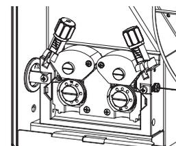
It is also possible to activate the wire feed via the torch trigger in this way:
