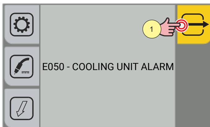
1. Press the [EXIT] key to repeat the torch filling procedure, until the alarm is no longer displayed.
