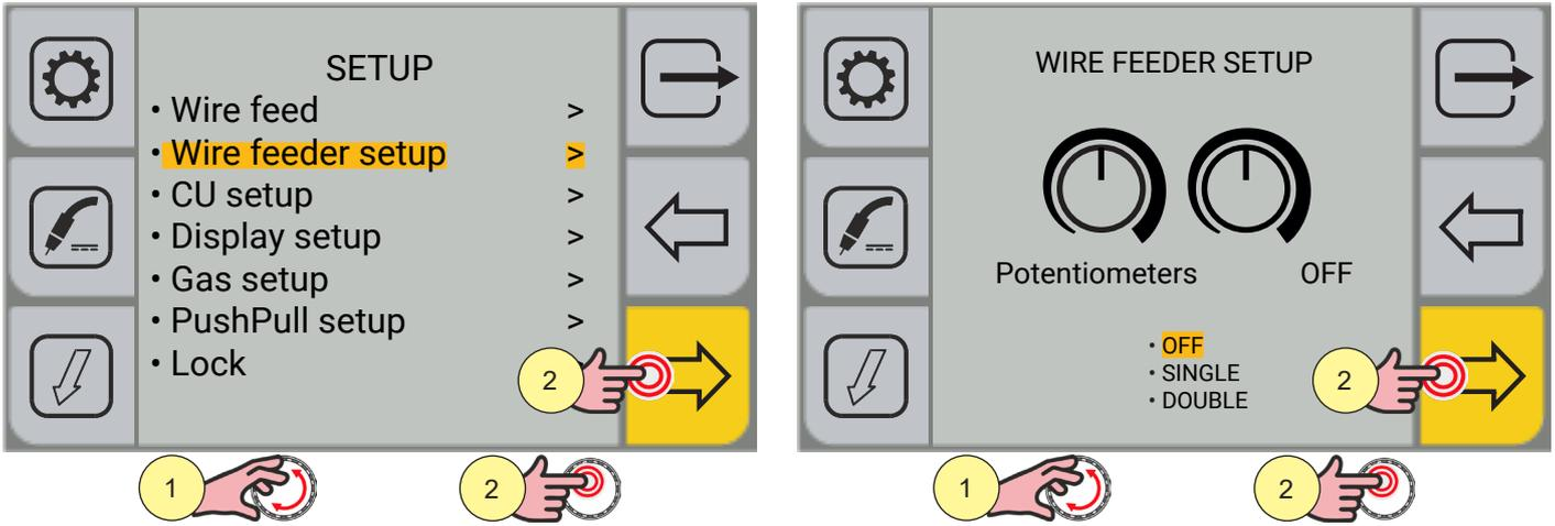
7. Turn the encoder to select the desired setting. Select the following path: Wire feeder setup>.
