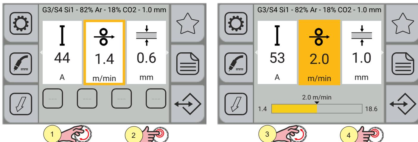
1. Turn the encoder to select the parameter to be changed; the selection is highlighted by a thicker border around the box.
