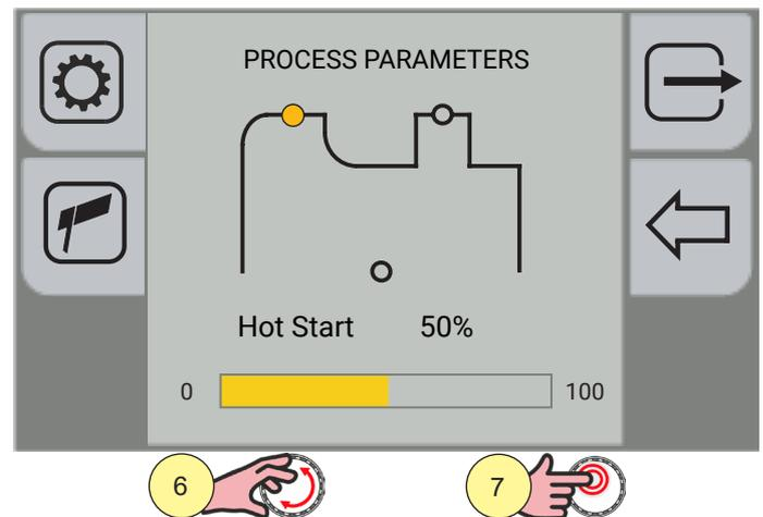
4. Turn the encoder to select the parameter to be modified.
