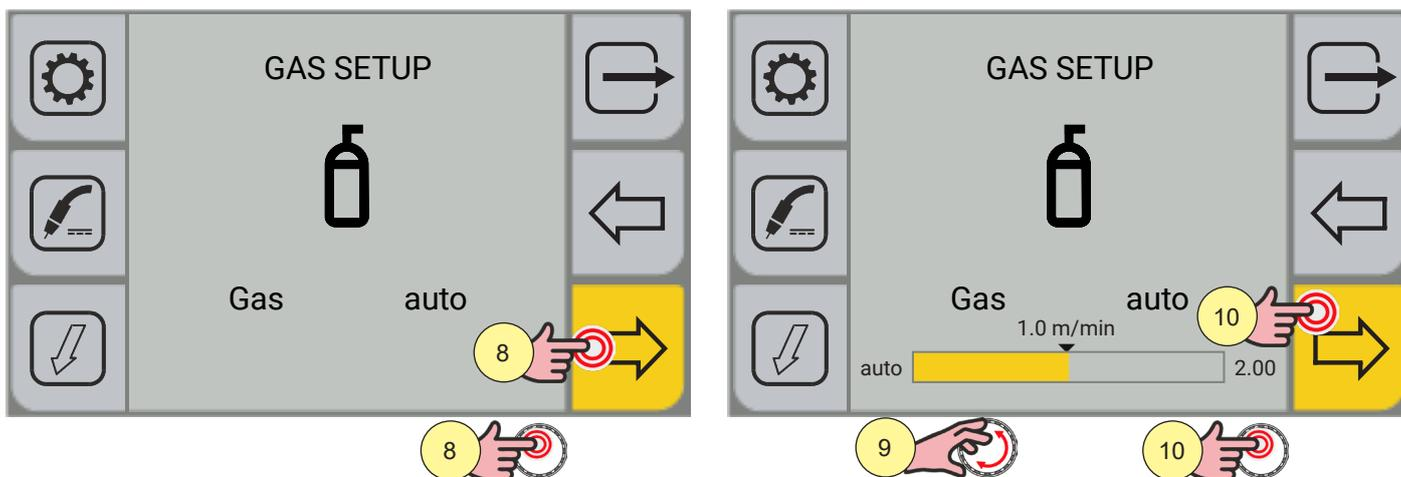
8. Press the [ENCODER] key to activate the parameter change.
