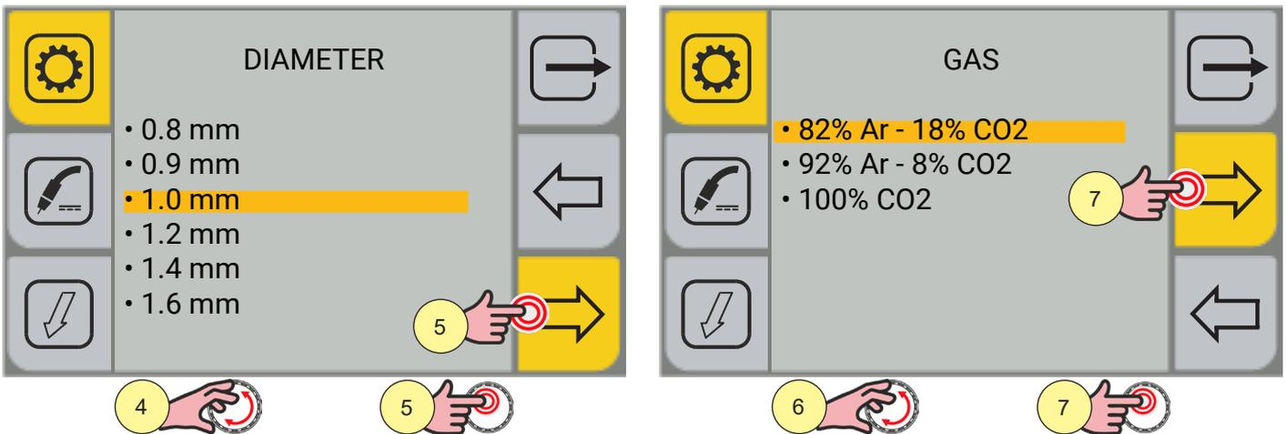
**DIAMETER:** allows you to select the diameter of the filler wire for welding. The available wire diameters depend on the material selected.
