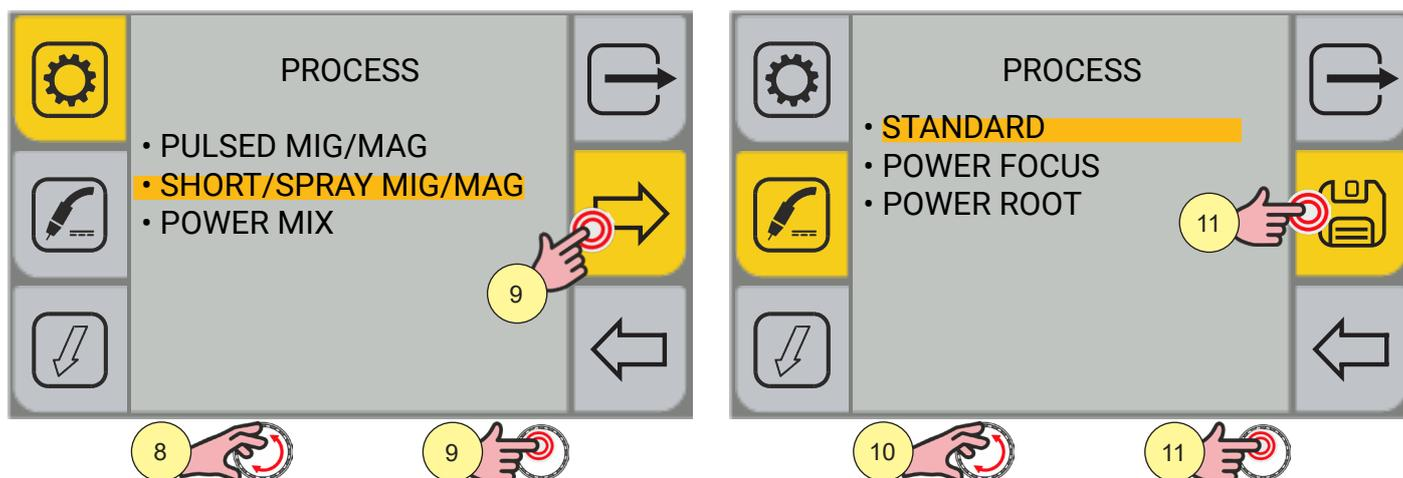
**PROCESS (1 LEVEL):** allows you to select only the welding processes compatible with the settings previously made.
