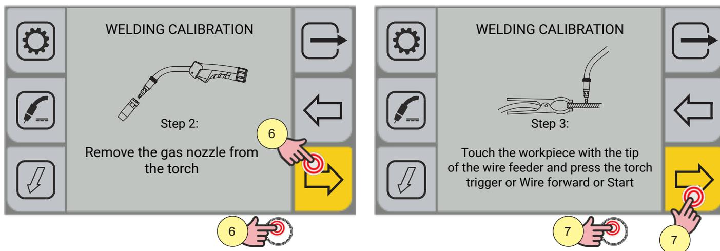
6. Press the encoder key or the [NEXT] key, or the torch trigger to confirm, or the [Wire forward] key.
