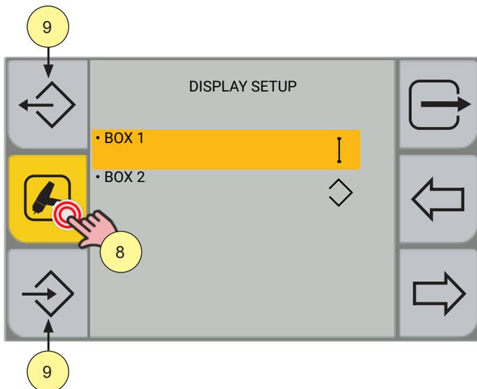
8. The display setup screen is linked to the welding process. Pressing the process selection key repeatedly scrolls through the different display setup screens of the various welding processes.
