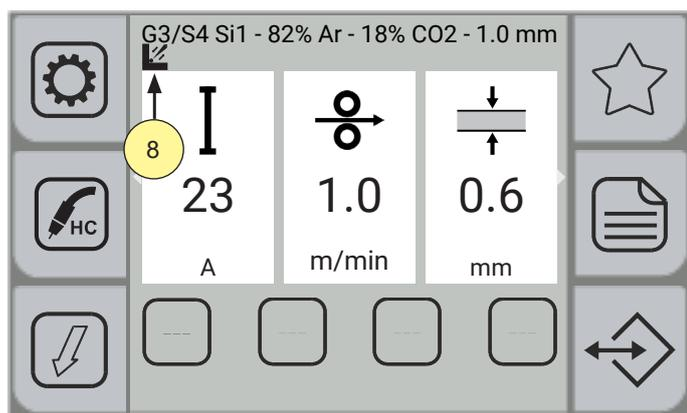
8. Below the wording of the synergic curve, the activated DSI procedure icon appears.
