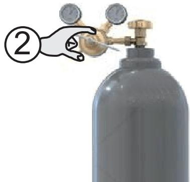
2. Regulate the pressure of the gas flowing from the torch by means of the flow meter connected to the gas cylinder.
